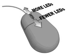
5. Adjust the mouse wheel until some of the LEDs are off, then move the mouse in a circular path (clockwise or counterclockwise). You should see the lighted LEDs rotate.
